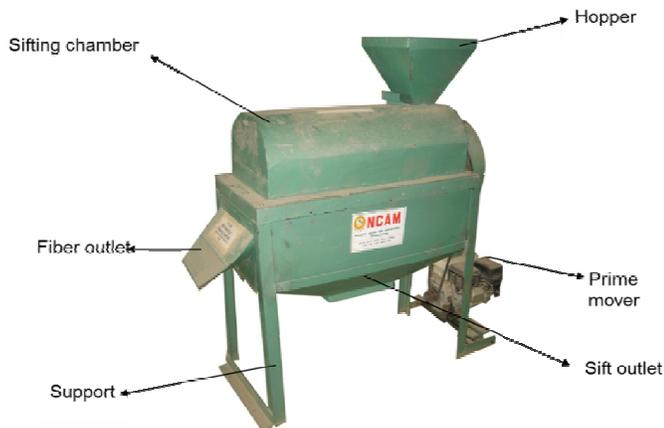
Figure 1. Pictorial view of the motorized sifter.
