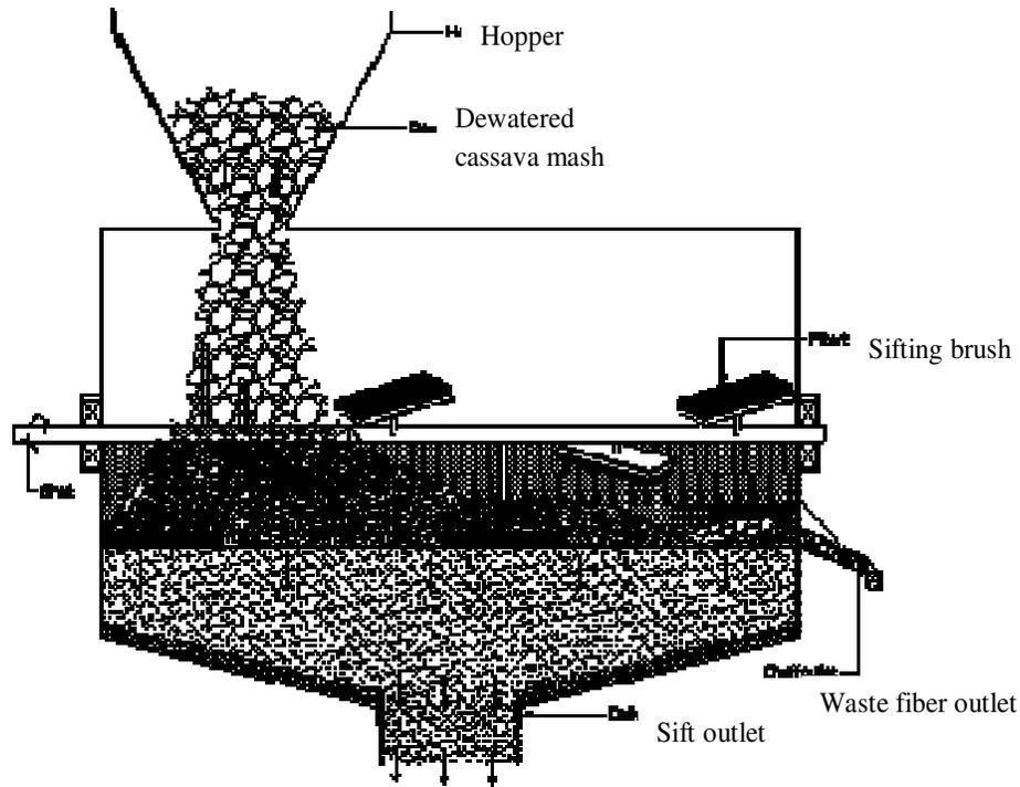
**Figure 3.** Sectional view of the sifter and material flow in the sifter.
