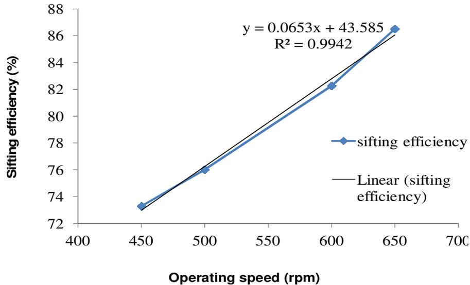
Figure 4. Effects of speed on sifting efficiency.
