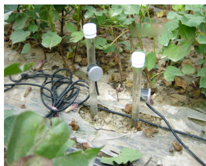
Figure 2. TS-2 negative pressure meter to measure soil water potential in the cotton field.
