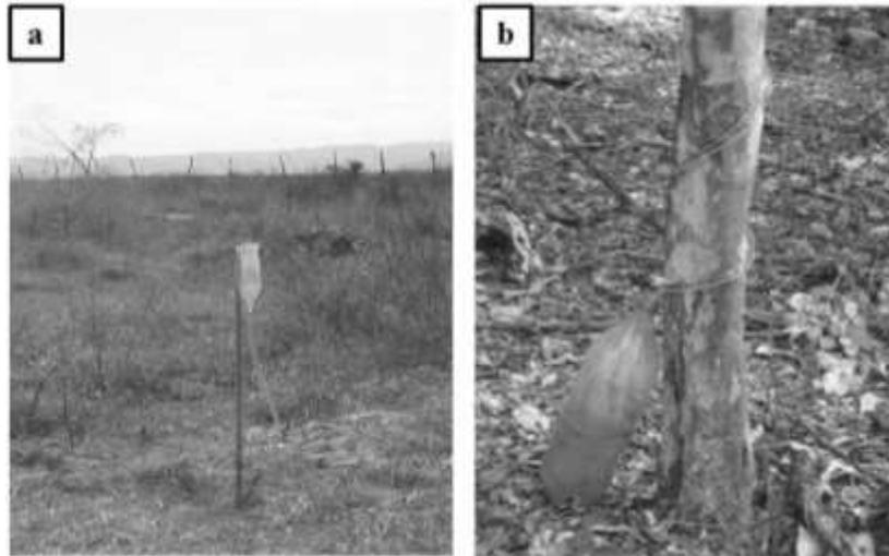
**Figure 1.** (a) Rainfall collector, (b) Stemflow collector.
