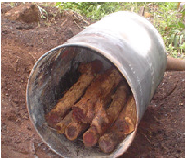
Figure 2. Partially filled drum kiln.
