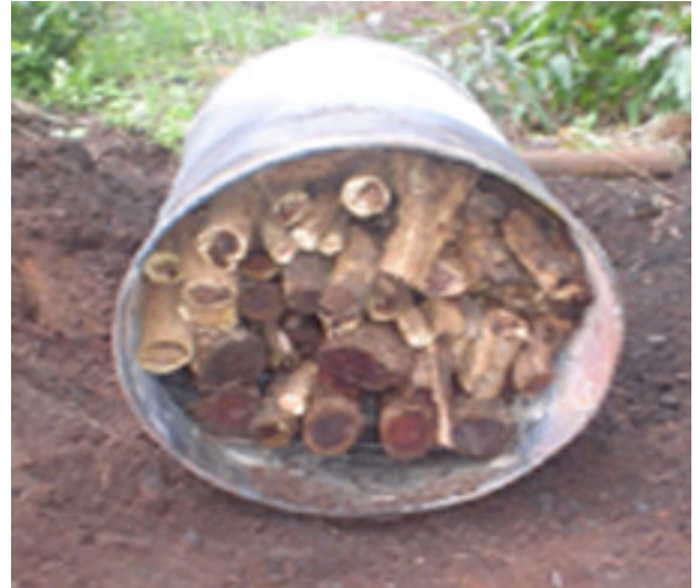
Figure 3. A fully loaded drum kiln.
