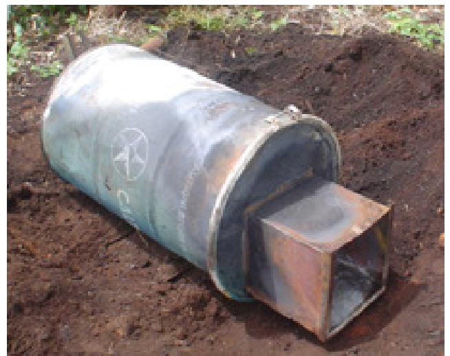
Figure 4. Loaded drum kiln closed with lid fitted with firing door.
