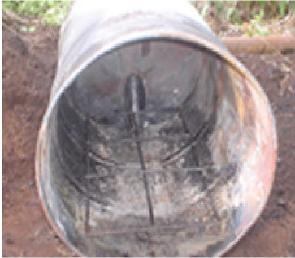
Figure 1. Empty (modified) drum kiln.
