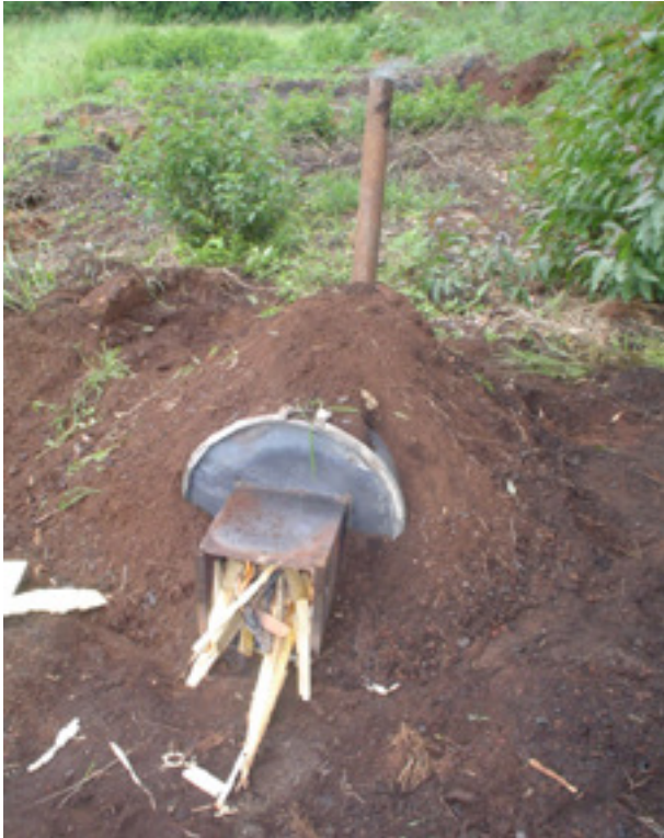
Figure 5. Small pieces of the firewood stacked at the firing section and lit.
