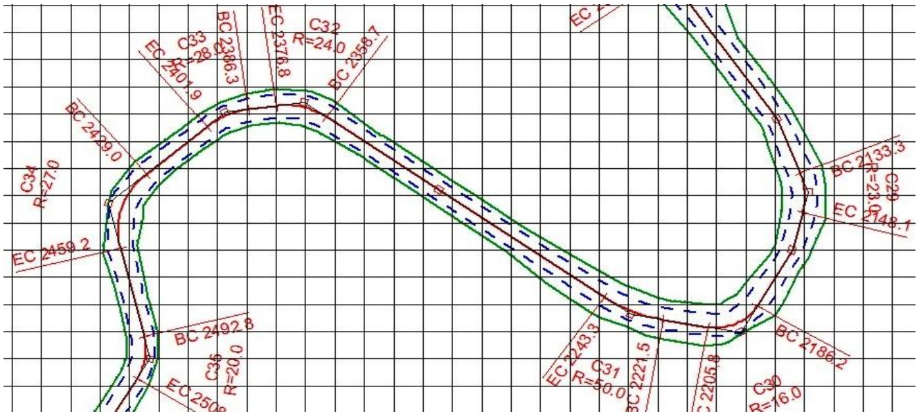
Figure 2. Designing forest road using RoadEng software.
