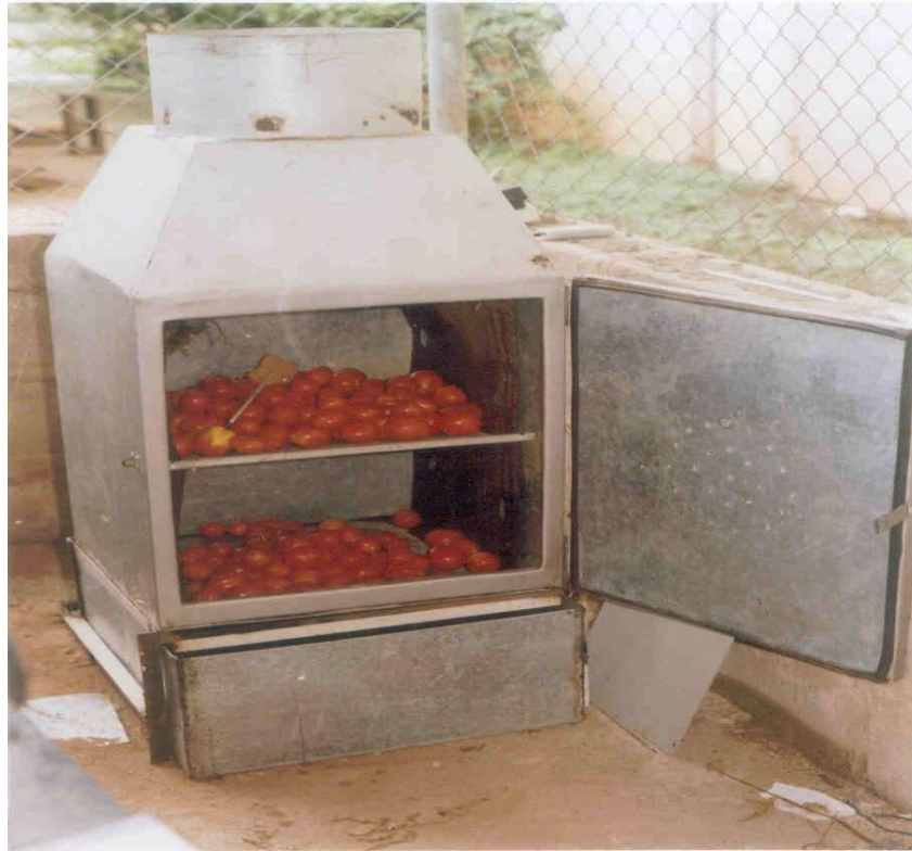
Figure 1a. Evaporative cooling system with the fresh tomatoes fruit.
