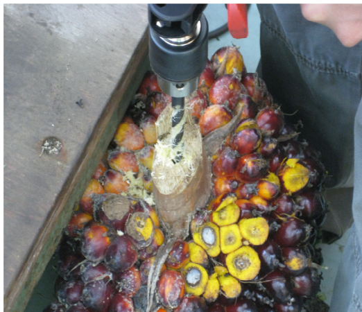
Figure 5. A hole drilled at the middle of the stalk using hand drill.
