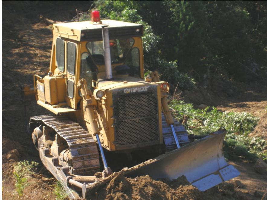
Figure 1. CAT D7G model bulldozer.
