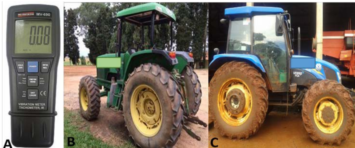
Figure 1. (A) Accelerometer of Instrutherm brand - MV690; (B) 4x2 TDA model without cabin manufactured in 1997 with engine nominal power of 89kW; (C) 4x2 TDA model with cabin manufactured in 2014 with engine nominal power of 65 kW (A). Source: http://www.instrutherm.com.br .
