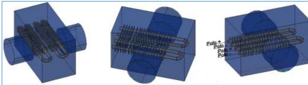
**Figure 2.** Device used to heat the grain mass.
