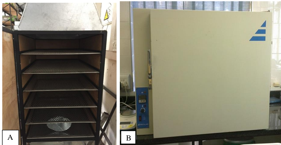
Figure 1. (a) Drying chamber of a modified naturally ventilated solar-venturi dryer and (b) hot air oven dryer. Source: Authors
