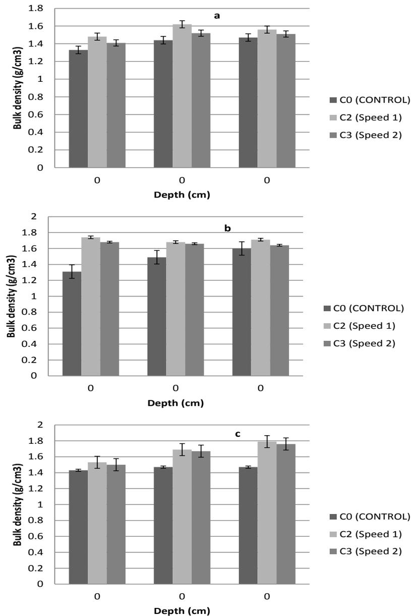
**Figure 1.** Bulk density for three level of compaction with varying the frequency of tractor passages (C0: no compaction, C1= speed 1 C2= speed 2) under three moisture conditions (a) H0 (t=0), (b) H1 (after 15 days), (c) H2 (after 30 days). The same type of tractor was used for all the treatments with a tyre inflation pressure of 1500 kg/cm<sup>2</sup>.
