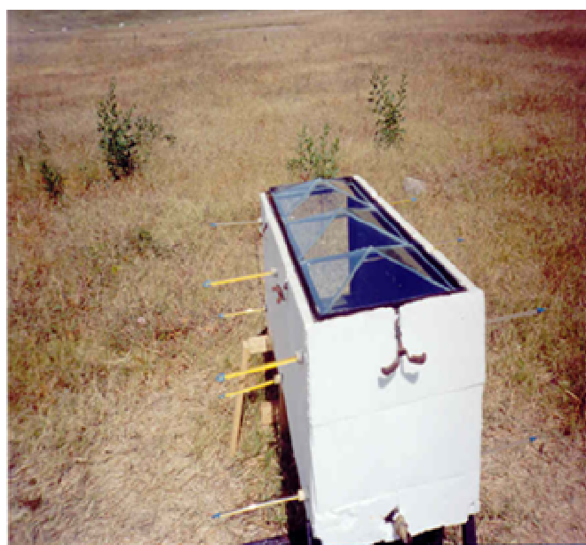
Figure 10. Prototype with modified pyramid-shaped glass cover.
