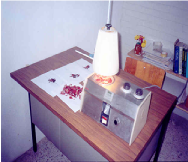
Figure 6. Determining Roselle drying properties using Thermobalance.
