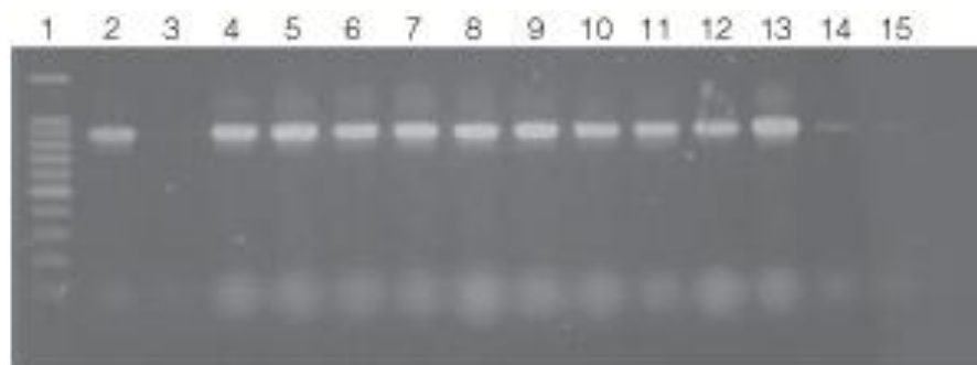
Figure 4. PCR amplifications of bacterial genomic DNA from various soil bacteria using the automated Biomek® 2000 protocol. The PCR DNA fragment is 875 bp. Lane 1, 100 bp DNA Ladder (Cat.# G2101); lane 2, E. coli JM109 positive control DNA isolated using manual protocol; lane 3, negative control no template; lanes 4 and 5, E. coli (Biomek® protocol); lanes 6 and 7, Enterobacter sp.; lanes 8 and 9, Azotobacter venelandi ; lanes 10 and 11, Rhizobium leguminosarum ; lanes 12 and 13 Acetobacter ; lanes 14 and 15 Citrobacter freundii . All bacteria were grown in ATCC 111 Rhizobium X Medium.
