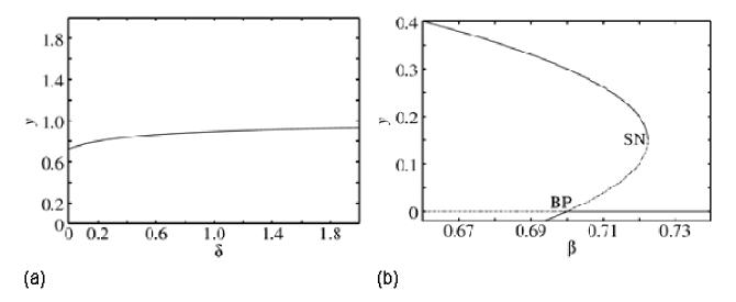
Figure 1. Bifurcation diagrams for Equation 5. a: Bifurcation with  $\delta$  as the control parameter,  $\beta = 0.2$ . Notice lack of sensitivity to  $\delta$ ; b: Stable and nonstable states with  $\delta = 0.7$ . Solid lines show stable steady states, dashed lines show unstable steady states. SN is the sadle node, BP is the bifurcation point (see text for explanation).
