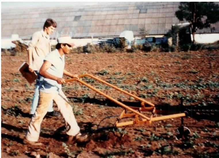
**Figure 2.** Prototype of the "chassis to keep implements" in field studies. (Source: author's file).
