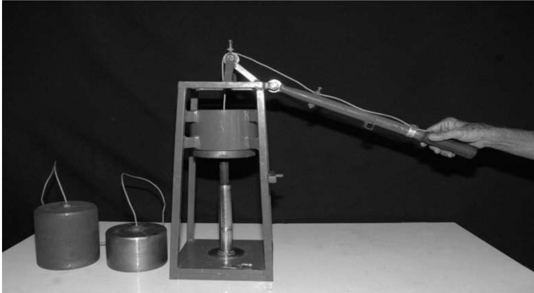
Figure 1. Compression treatment: from left to right: 13.2 and 8.8 kg weights; iron structure with 4.4 kg weight inside, lever for compression control, wooden stick to compress wheat grains, 15.30 ml microchondrometer with cutter bar blade in front.
