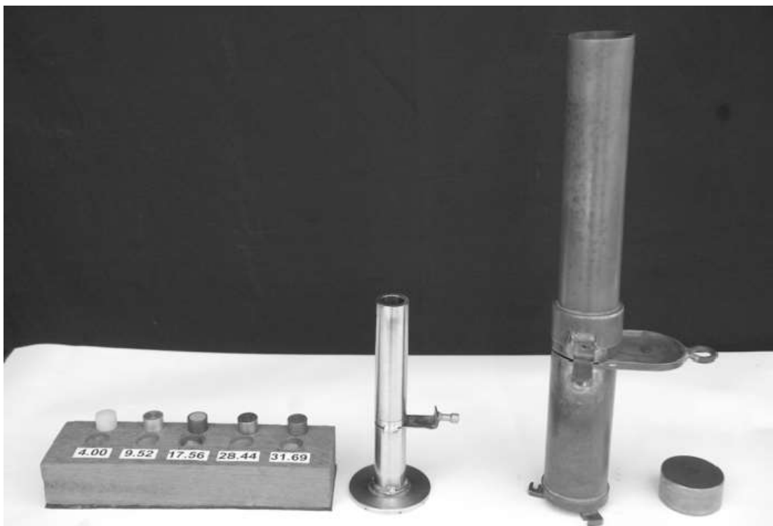
Figure 2. From left to right: Five pistons weight used in the 15.30 ml microchondrometer and the 250 ml chondrometer with its piston.
