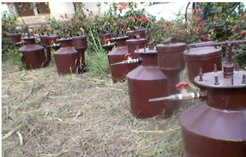
Figure 1. The metallic digesters used for the Research at Biotechnology Research Center, Nnamdi Azikiwe University Awka, Nigeria.
