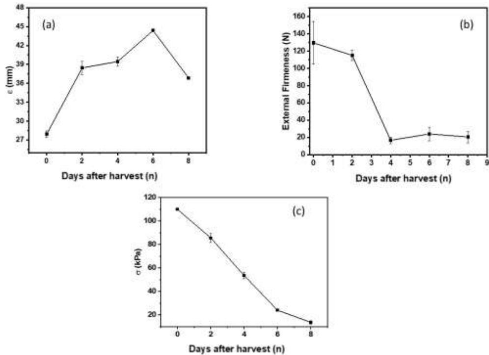
**Figure 3.** Mechanical assays of *Papayas* as a function of number of days after harvest: (a) external firmness, (b) deformation and (c) Henck tension. The error bar represents the deviation from medium value calculated from experiments in four different fruit per day.
