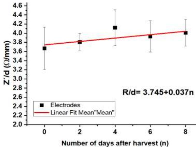
**Figure 4.** Dependence of real part of impedance of papaya (at 1 MHz) as a function of ripening degree. The error bar represents the deviation from medium value calculated from experiments in four different fruit per day.
