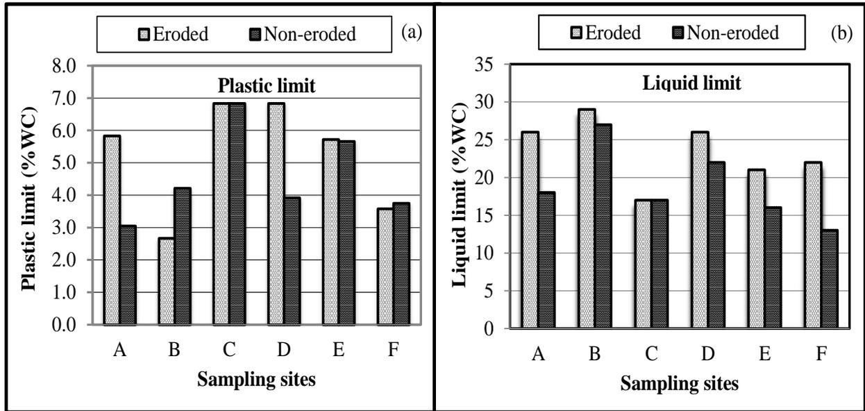
Figure 3. The plastic limit (a) and liquid limit (b) for both eroded and non-eroded areas.
