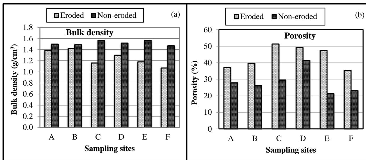
**Figure 2.** Soil bulk density (a) and porosity (b) for eroded and non-eroded sites.
