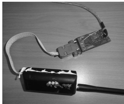
Figure 5. Picture of the sealed WUSN node.
