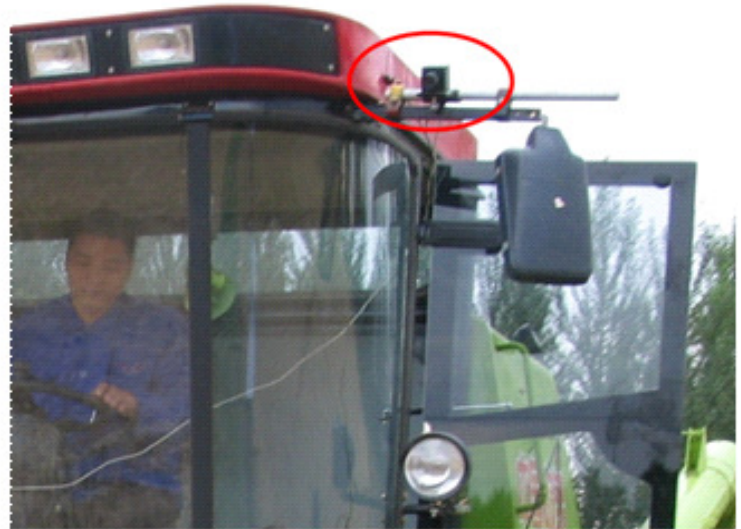
Figure 1. Camera installation and coordinate systems, the right are the combine harvester platform.
