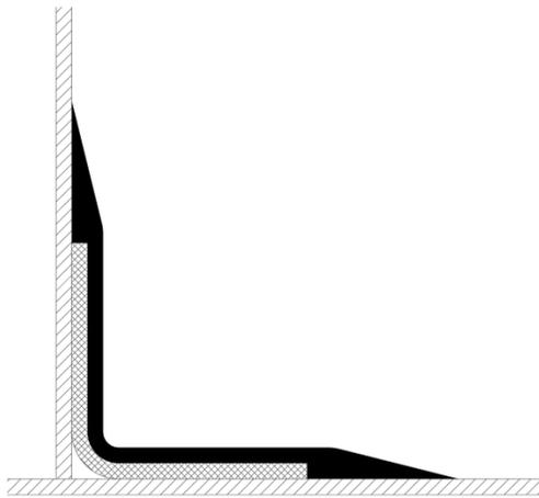
**Figure 4.** Joints ribbon-bitumen sealing.
