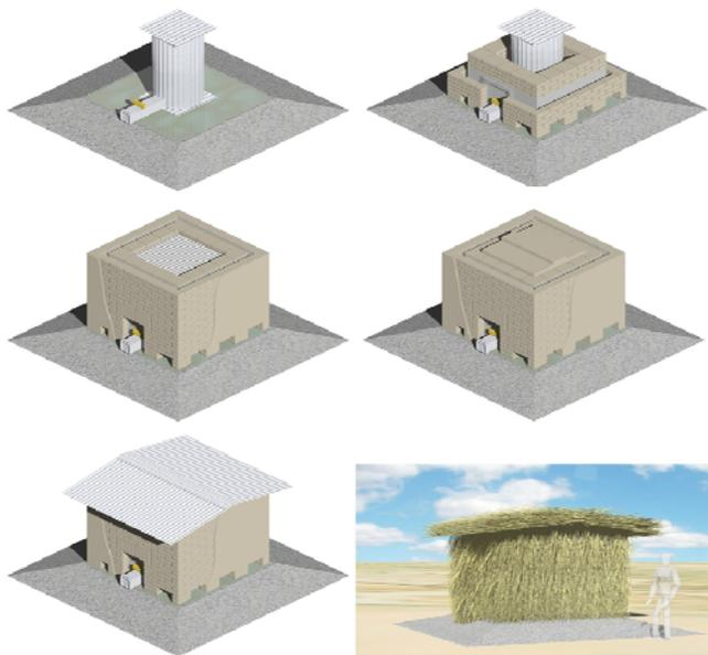
Figure 6. Phases of the silo completion (type A).
