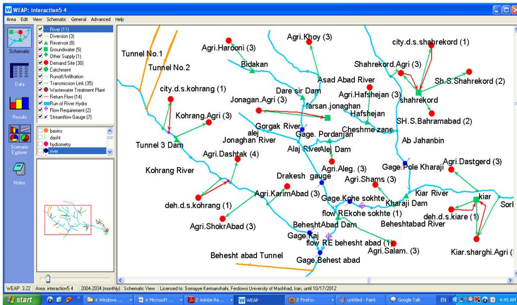
Figure 2. Configuration schematic of water resources system of Behesht Abad and Kuhrang basins.
