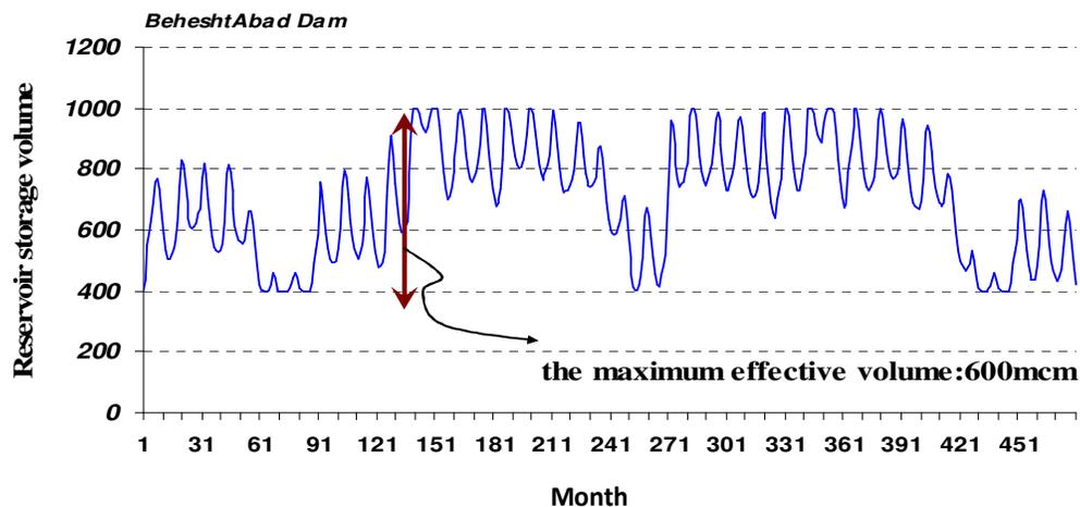
**Figure 6.** Changes in the water storage volume in the reservoir of Behesht Abad Dam in different months of simulation.
