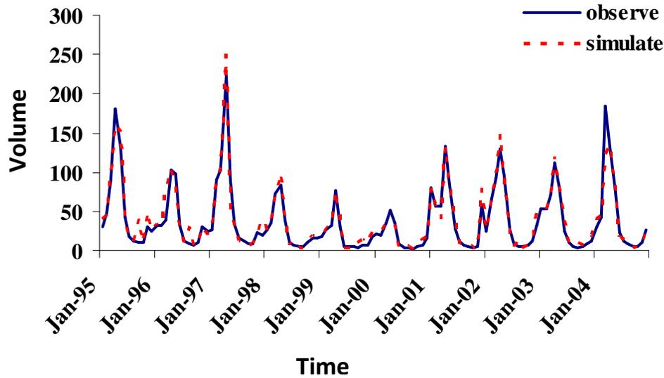
Figure 3. Observed and calculated monthly discharge.
