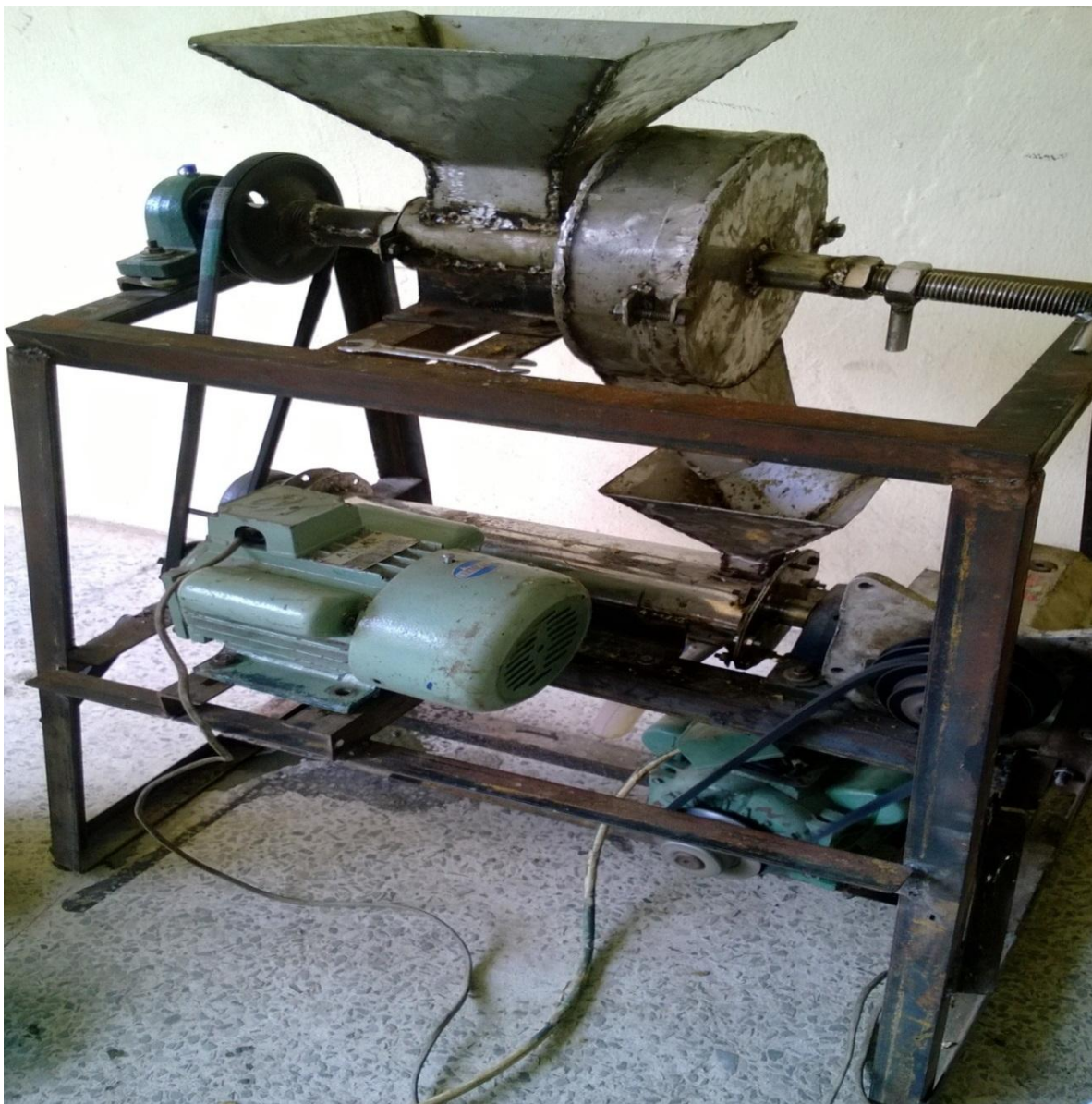
Figure 2. The developed motorized ginger juice expression machine.
