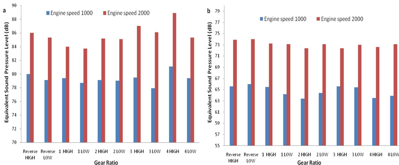
Figure 5. Sound pressure level values at MF tractor while it was moving by different gears and engine speed (1000 and 2000 rpm) (a) at right ear of driver, and (b) at surroundings (L and H stand for low and high gears).
