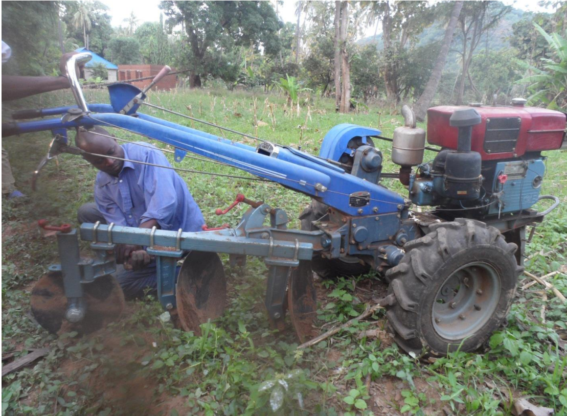
Figure 1. Disc plough setting for tillage operation. Source: Author
