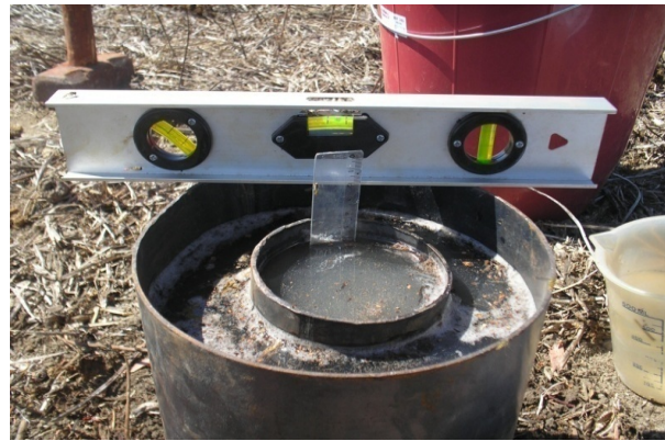
Figure 5. Installation of the double-ring infiltrometer.
