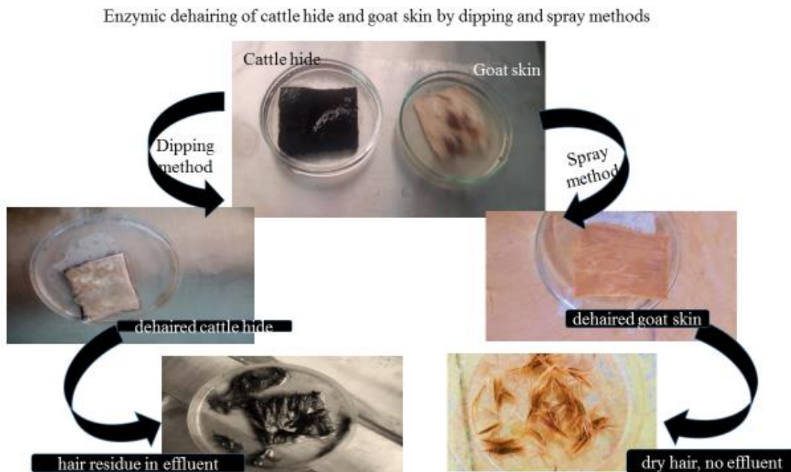
Figure 10. Difference in application of dehairing method on quality of hide and skin.
