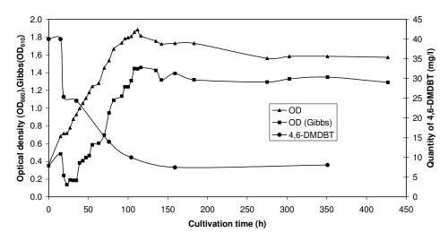
Figure 5. Time course of 4, 6-DMDBT desulfurization at 30 °C by growing cells of RIPI-S81.
