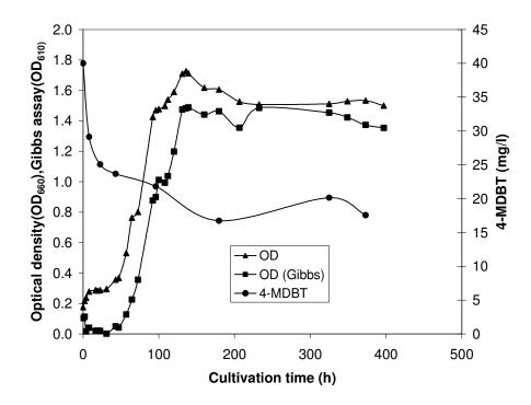
Figure 6. Time course of 4-MDBT desulfurization at 30 °C by growing cells of RIPI-S81.
