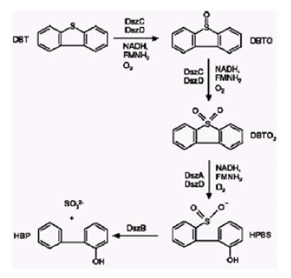
Figure 1. Proposed pathway of DBT- desulfurizing by several bacteria including *RIPI-S81*.
