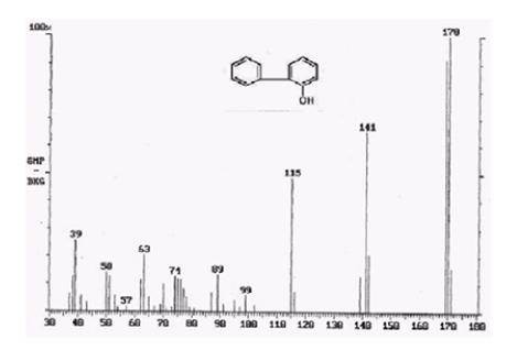
**Figure 2.** GC-MS spectrum of the DBT final metabolite with strain *RIPI-S81*. This metabolite was identified as 2-HBP.
