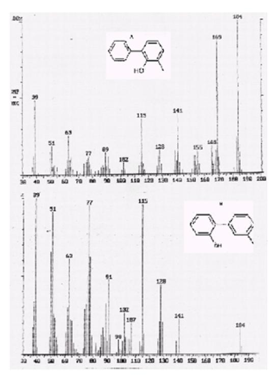
**Figure 4.** GC-MS spectrum of the final metabolites with strain *RIPI-S81*. These metabolites were identified as, A: 2-hydroxy-3-methyl-biphenyl & B: 2-hydroxy-3'-methyl-biphenyl (2-HMBP).
