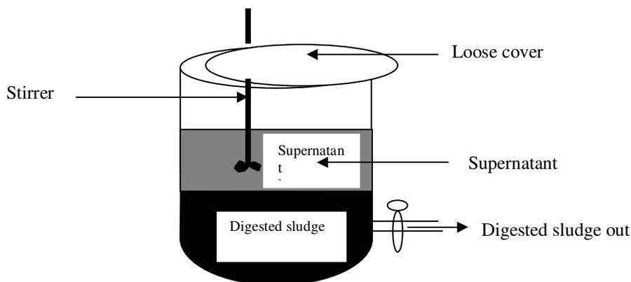
Figure 2. Laboratory apparatus for conducting aerobic digestion studies.
