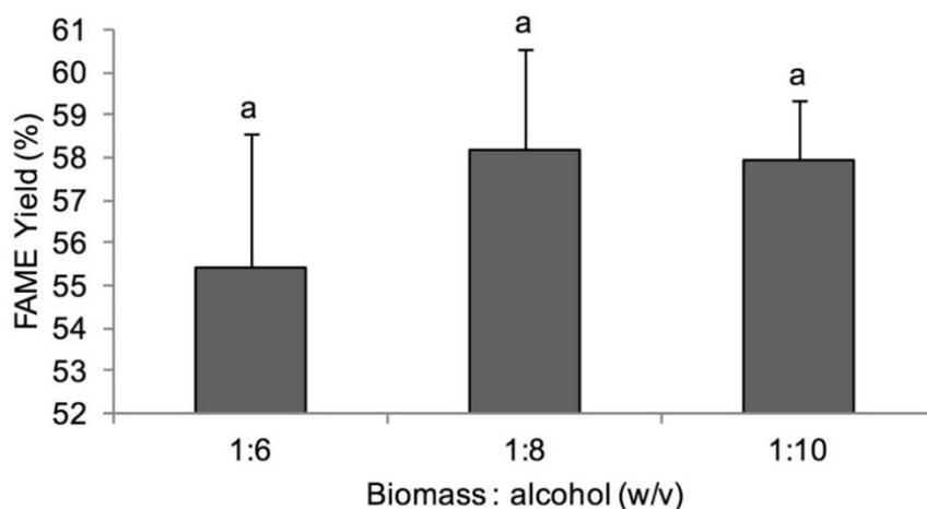
**Figure 2.** Influence of the biomass : alcohol ratio on biodiesel yield (at 90°C for 90 min using 60% wt. H<sub>2</sub>SO<sub>4</sub>). Averages with different indices are significantly different ( $p < 0.05$ ).
