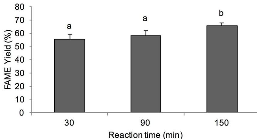
**Figure 4.** Influence of reaction time on biodiesel yield (at 90°C using biomass to methanol ratio of 1:8, 60% wt. H<sub>2</sub>SO<sub>4</sub>). Averages with different indices are significantly different ( $p < 0.05$ ).
