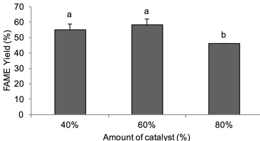
**Figure 3.** Influence of the catalyst concentration on biodiesel yield (at 90°C for 90 min using biomass to methanol ratio of 1:8). Averages with different indices are significantly different ( $p < 0.05$ ).
