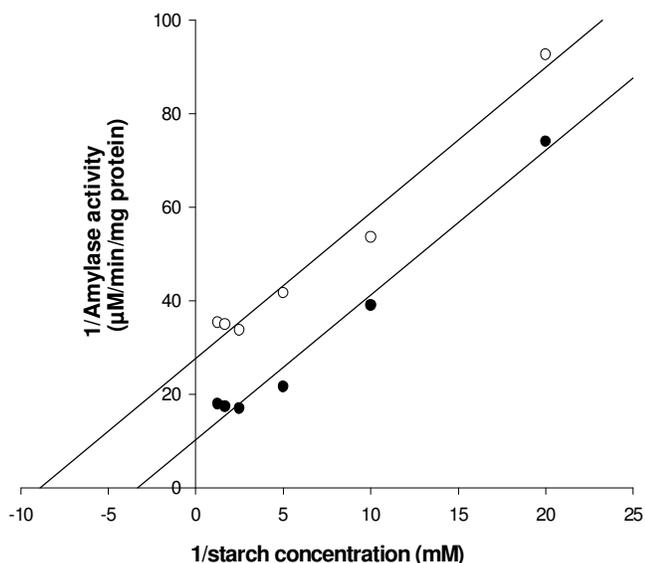
**Figure 7.** Double reciprocal plot (Lineweaver-Burk plots) of enzyme activity (velocity) versus starch concentration (%) to obtain values for the maximum velocity ( $V_{max}$ ) and Michaelis constant ( $K_m$ ) for gut amylase (blank circles) and salivary amylase (filled circles).
