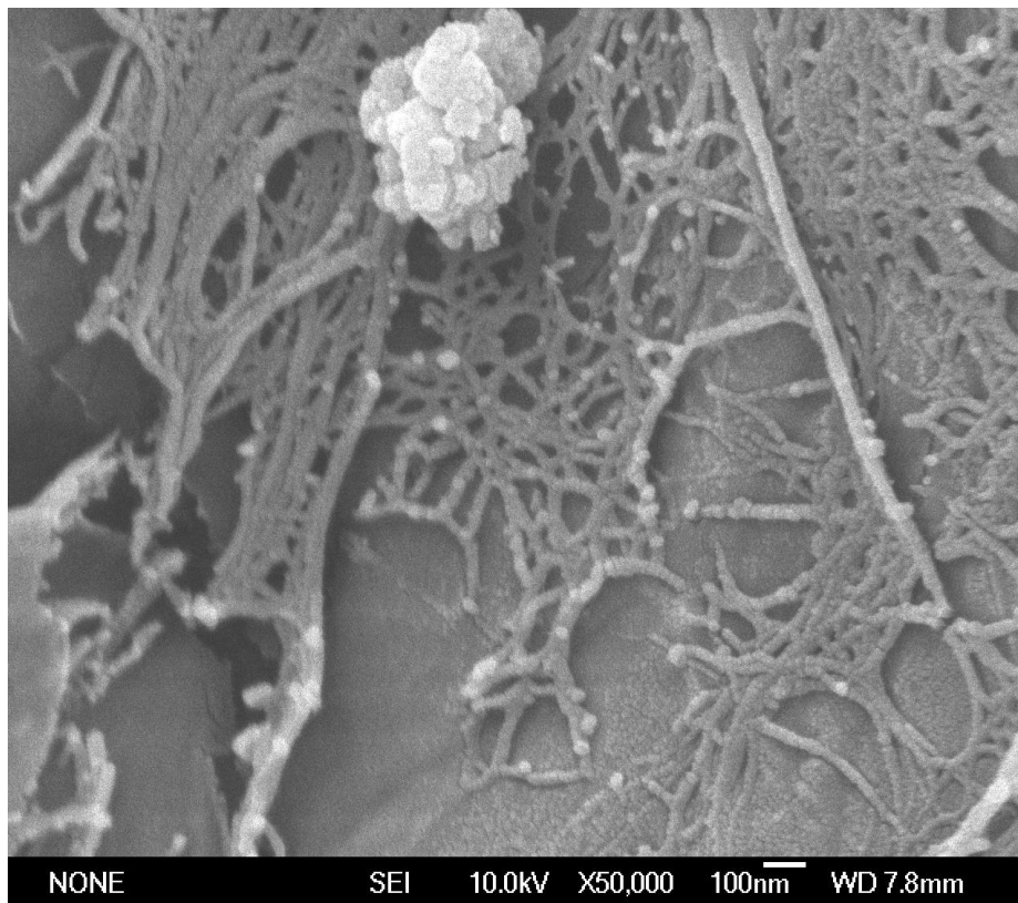
Figure 5. Nano-structure of gelatin at 100 nm pretreated with acetic acid, NaOH and NaCl.
