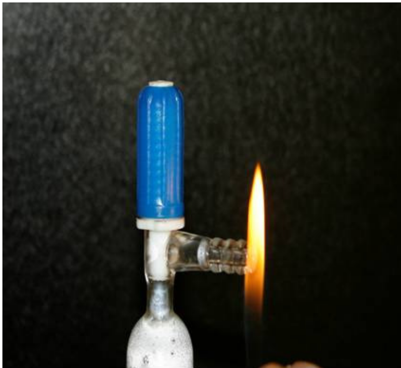
Figure 9. Burning of photo catalytically produced methane.
