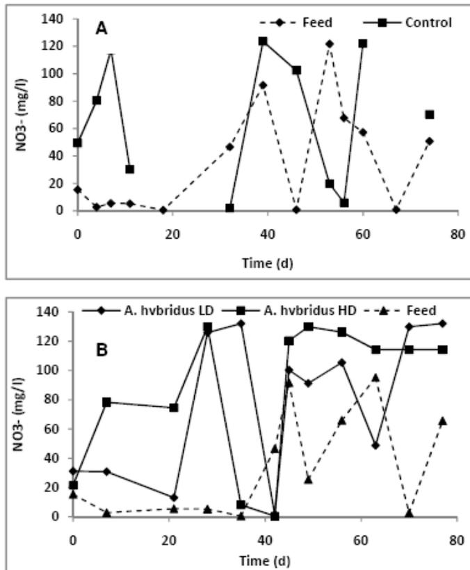
**Figure 7.** Profiles of NO<sub>3</sub><sup>-</sup> in raw wastewater (feed), filtrates of control (A) and the planted beds (B) with *A. hybridus* at low and high densities.
