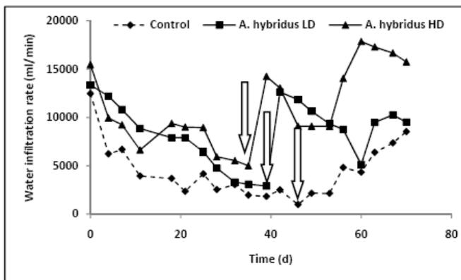
**Figure 3.** Water infiltration rates profiles in the control and planted beds with *A. hybridus* at low (LD) and high (HD) densities. The arrows indicate the period of solids removal on the bed surface
