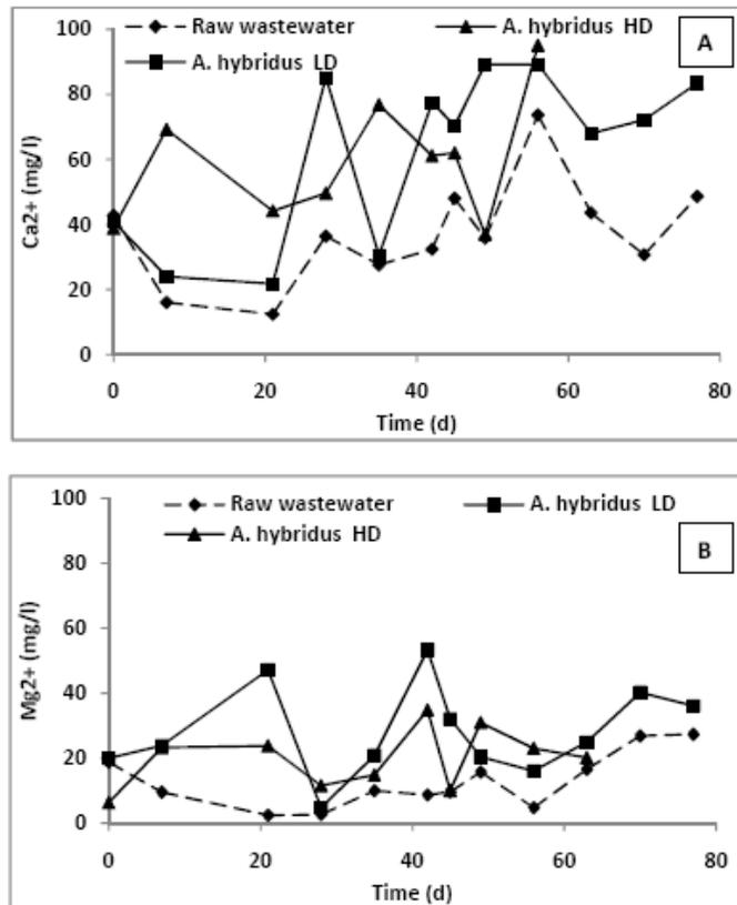
**Figure 10.** Profiles of Ca<sup>2+</sup> (A) and Mg<sup>2+</sup> (B) in the raw wastewater (feed), the filtrates of the planted beds with *A. hybridus* at low (LD) and high (HD) densities.
