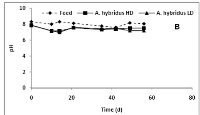
**Figure 4.** pH profiles in the raw wastewater and in the filtrates of the control (A) and the planted beds (B) with *A. hybridus* at low (LD) and high (HD) densities.
