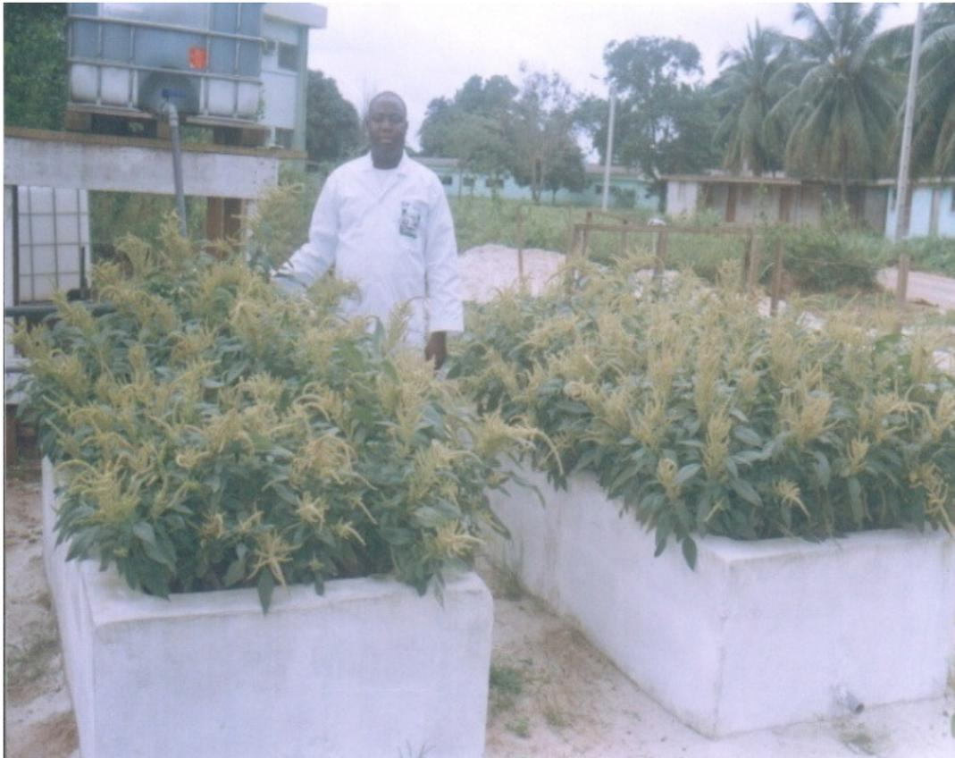
**Figure 1.** Photograph of two vertical completely drained planted beds with *A. hybridus*.
