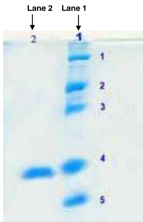
Figure 3. SDS page of xylanase. Lane 1, molecular weight markers; Lane 2, purified enzyme. Molecular marker includes the following proteins, 1, Myosin (205,000 Da); 2, phosphorylase b (97,400 Da); 3, bovine serum albumin (66,000 Da); 4, ovalbumin (43,000 Da); 5, carbonic anhydrase (29,000 Da).
