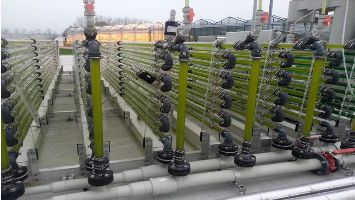
**Figure 6.** Photograph of a Horizontal Tubular Reactor (HTR) (taken in November 2013; AlgaePARC, Wageningen University). HTRs are composed of horizontal transparent glass or plastic (polyethylene) tubing. Gas transfer takes place in the tube connection or via a dedicated gas-exchange unit, and the angle toward sunlight is particularly adequate for efficient light harvesting (Carvalho et al., 2006).
