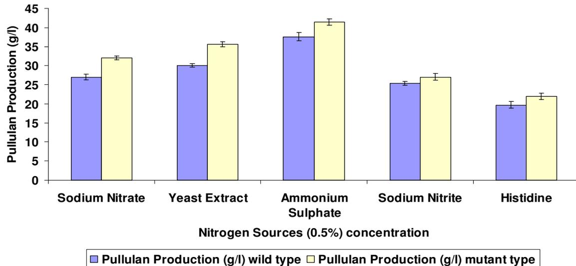
Figure 6. Effect of different nitrogen sources on pullulan production.
