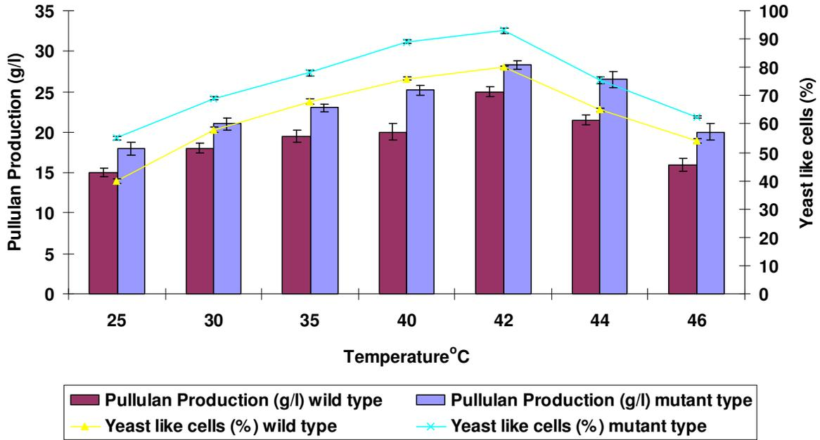
Figure 2. Effect of temperature on production of pullulan and percentage of Yeast like cells.
