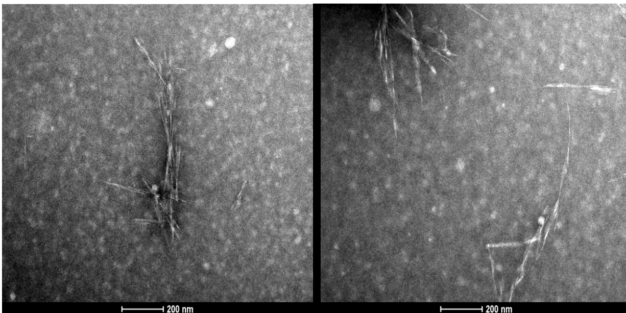
Figure 1. Micrographs obtained (TEM) from the coconut nanocellulose solution, evidencing the presence of nanocrystals (Scales: 200 nm).
