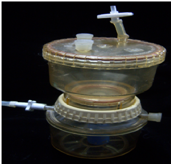
Figure 1. Nalgene® polysulfone filtration system modified as temporary immersion system.
