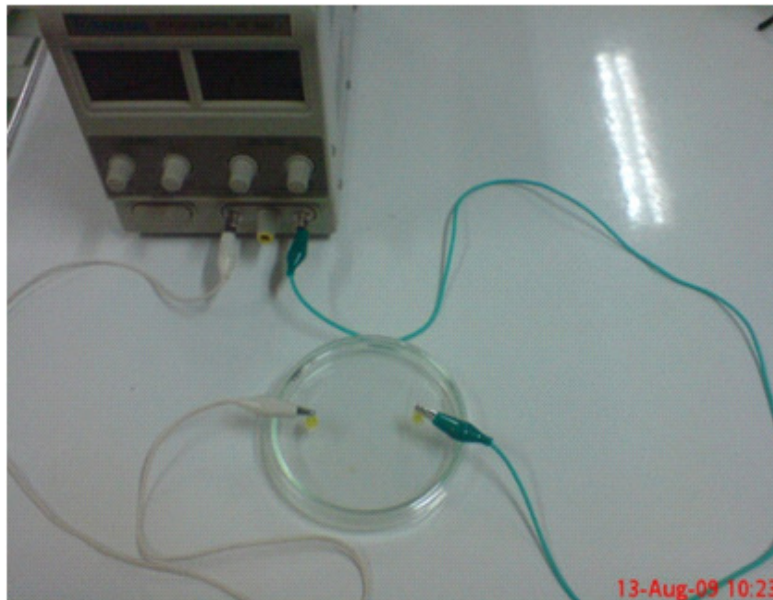
Figure 1. Experimental setup, glass petri dish with stainless-steel electrodes connected to DC power supply before placement into incubator
