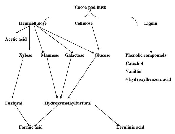
Figure 5. Reactions occurring during the hydrolysis of lignocellulosic materials. Source: Igbinadolor, 2012.
