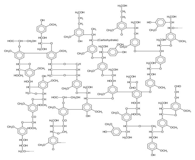
Figure 4. Lignin structure (Adapted from htpp:// www.en.wikilpedia.org/wiki/lignin).
