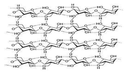
Figure 3. A strand of cellulose, showing the hydrogen bonds (dashed) within and between cellulose molecules (adapted from http://www.en.wikipedia.org/wiki/cellulose).
