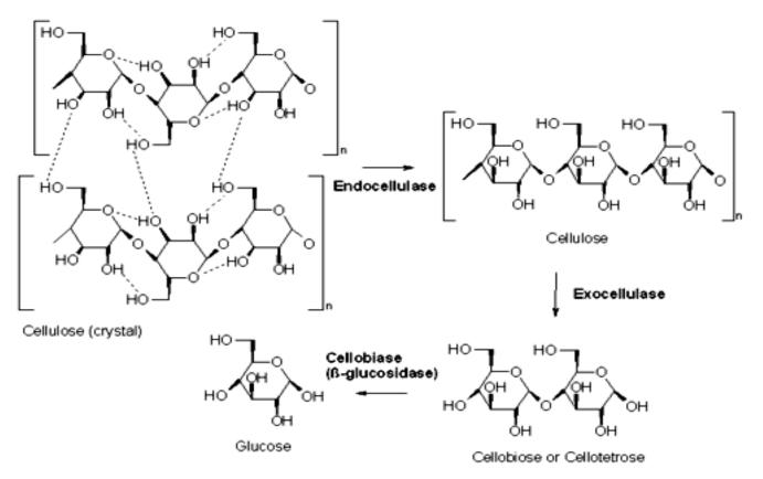
**Figure 6.** The 3 types of reaction catalysed by cellulases. Breakage of the non-covalent interactions present in the crystalline structure of cellulose (endo-cellulase) 2. Hydrolysis of the individual cellulose fibres to break into smaller sugars (exocellulases) 3. Hydrolysis of disaccharides and tetrasaccharides into glucose (beta-glucosidase) (adapted from http://www.en.wikilpedia.org/wiki/cellulose).
