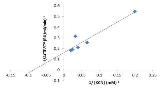
Figure 2. Lineweaver-Burk plot for *P. brazzeana* root rhodanese using KCN as substrate.
