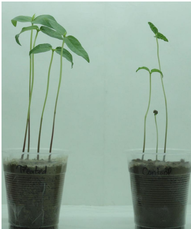
Figure 7. The growth of Vigna radiata in dye treated wastewater indicates that P. ostreatus treated wastewater is safe for plant growth.
