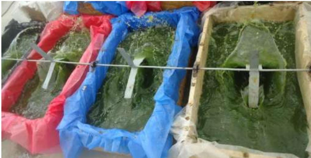
**Figure 3.** Aeration by modified rotating paddle wheel.
