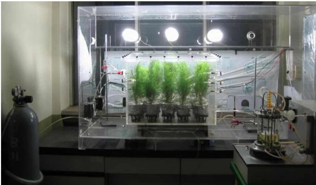
Figure 1. Schematic diagram (A) and photo (B) of the plant-based air filter system: 1, compressed air; 2, gas flow meter; 3, air filter; 4, fluorescent lamp; 5, C. macrocarpa ; 6, aluminum foil; 7, watering pipe; 8, water drain; 9, air bypass line; 10, bioreactor (flask or fermentor); 11, solid-phase microextraction; 12, medium in (only available in the chemostatic culture); 13, medium out (only available in the chemostatic culture); 14, peristaltic pump.
