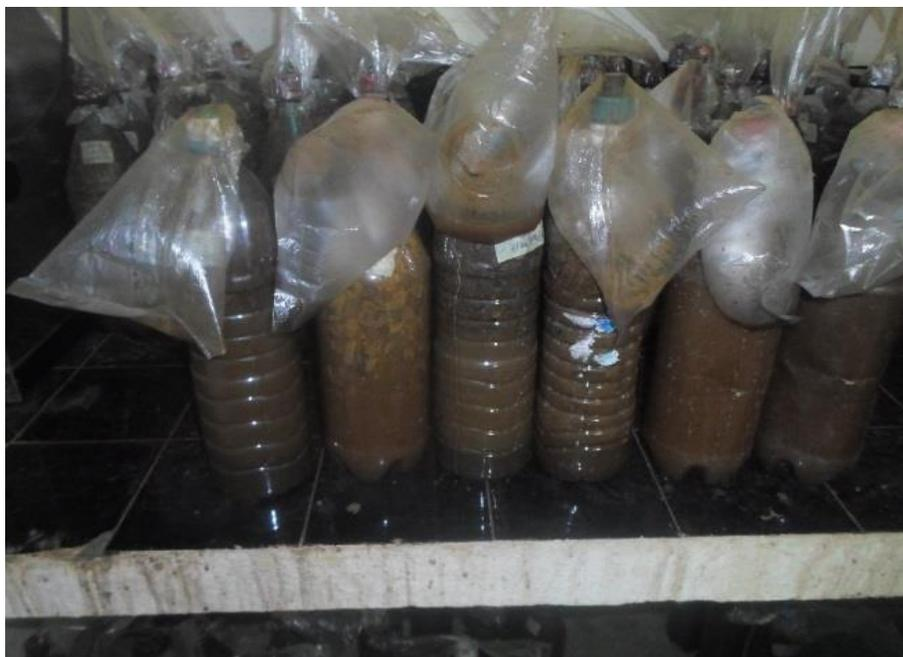
**Figure 1.** Mini-bioreactors producing biogas from dead neem leaves.
