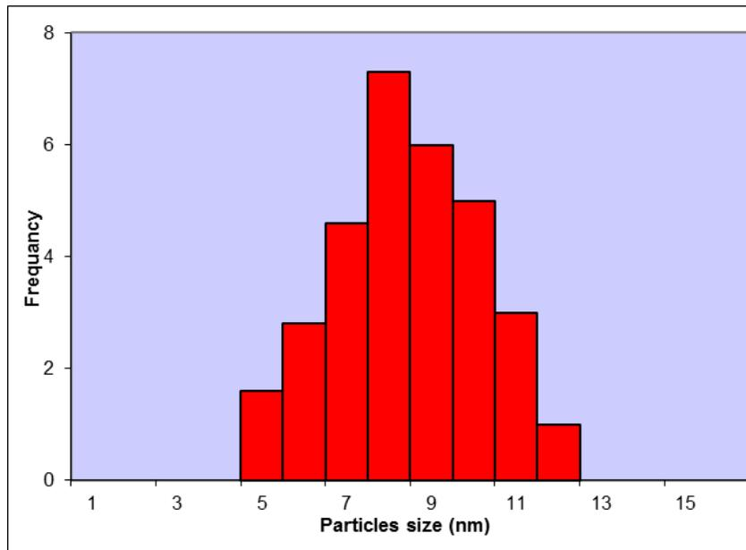
Figure 3. Particles size distribution of synthesized iron nanoparticles.
