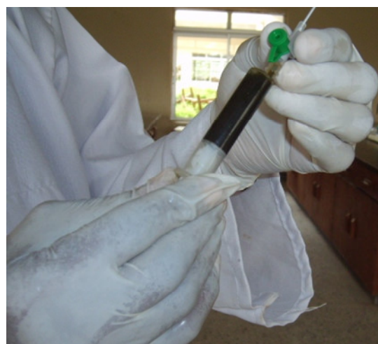
Figure 3. Connect the Mediflon intravenous cannula to the 10 ml syringe containing the test solution.
